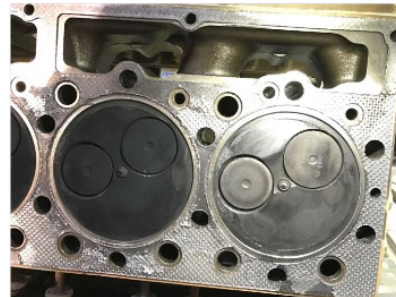
CAT 972G Loader Engine Disarmed, 10,000 hrs maintenance (3,000 hrs using FEROX by RENNSLI)
