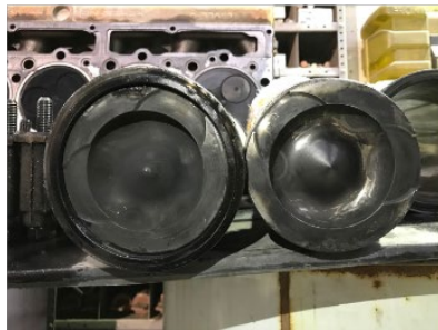
CAT 972G Loader Engine Disarmed, 10,000 hrs maintenance (3,000 hrs using FEROX by RENNSLI)
