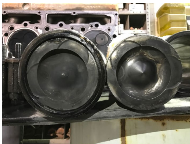
CAT 972G Loader Engine Disarmed, 10,000 hrs maintenance (3,000 hrs using FEROX by RENNSLI)
