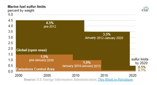
Vessel operators also have several choices for compliance with the new IMO sulfur limits. For example, IMO regulations allow for the installation of scrubbers, which remove pollutants from ships' exhaust, allowing them to continue to use higher sulfur fuels.
